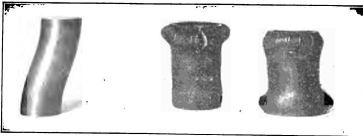
Fig. 33. — Metal in Compression.
